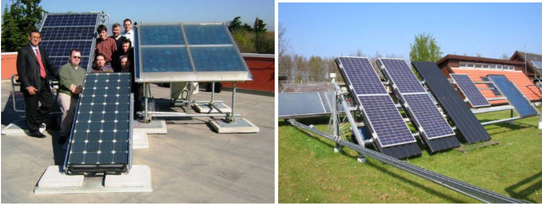
Figure 2: (a) PV/T testing site in Padova, visited by a number of IEA SHC Task 35 members, (b) PV/T testing site at the Danish Technological Institute with PV-Solarwall collectors.
